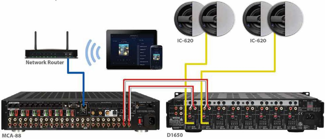
Using Bus input to share a source with multiple zones
